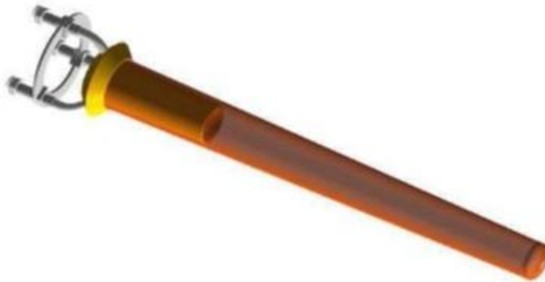
Figure 2.20. Conical liquid deuterium target used for the eg3 run period, measuring 40 cm in length, and the 4cm in diameter at its widest. The beam axis runs along the center of the target. The entrance and exit windows of the target cell were made with thin aluminum.
