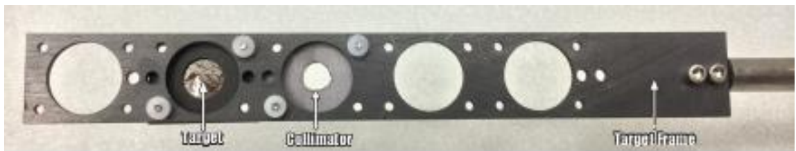
Figure 3.2 The carbon target ladder shown with a target frame, and collimator. The collimator is made out of tantalum and was used for beam tuning. All calibration sources were mounted on the same ladder to insure centering in the ICEBALL array.
