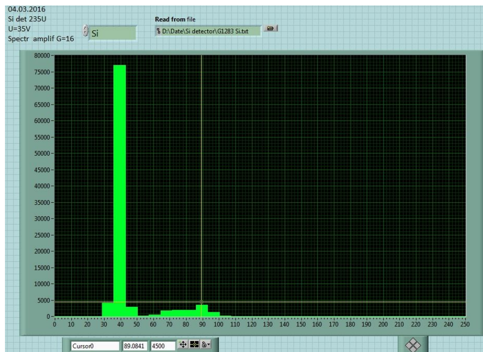
Fig. 21 The energy spectra of Si semiconductor detector from ^{235}\text{U} source
