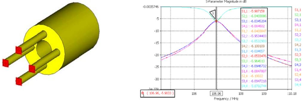
**Fig 21.** Response of the S parameters obtained from the simulation for a cavity with four input ports.
