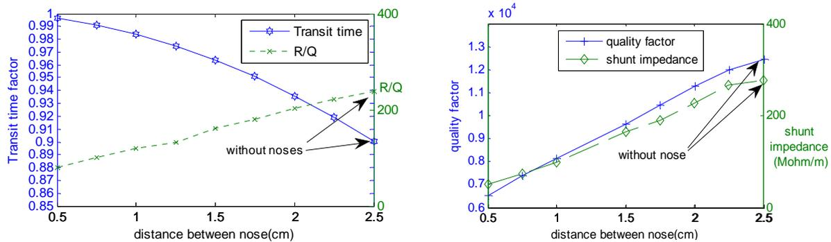
**Fig3.** Effects of nose gap size on various parameters of a linear accelerator.
