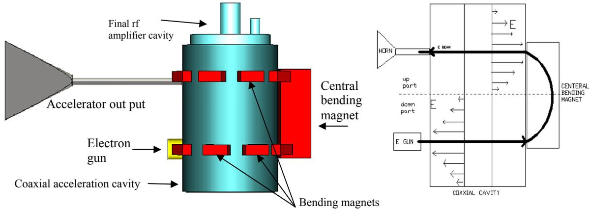
**Fig 13.** Section-cut view of the conceptual designed accelerator.
