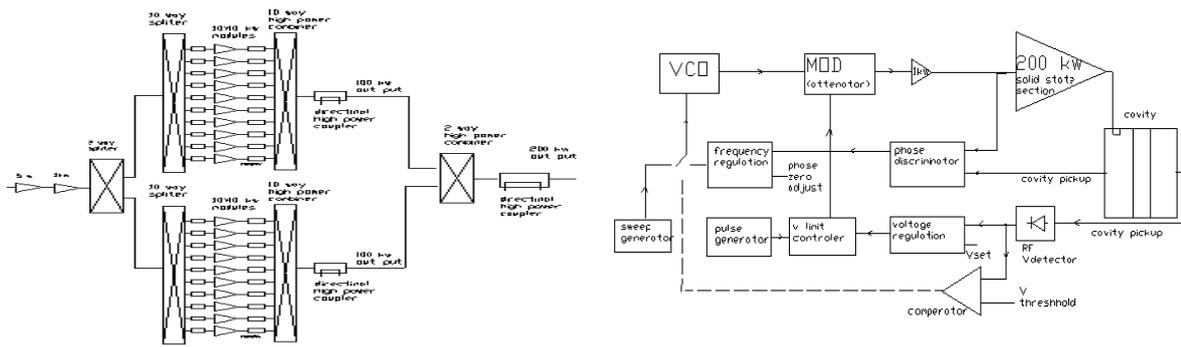
**Fig14.** Schematic sketch of a 200 kW RF system with a transistor amplifier for a Rhodotron accelerator.
