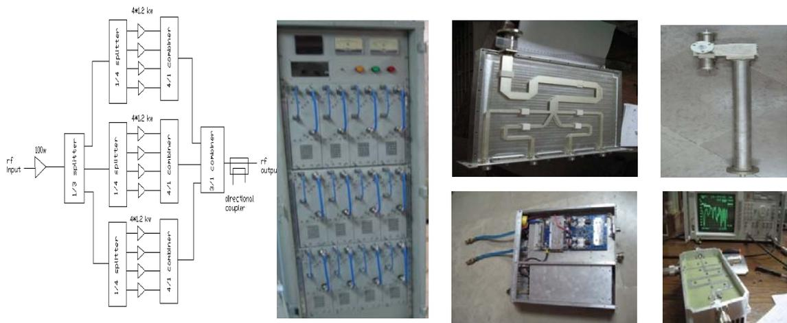
**Fig15.** the block diagram and some components of our 10 kW solid state amplifier .
