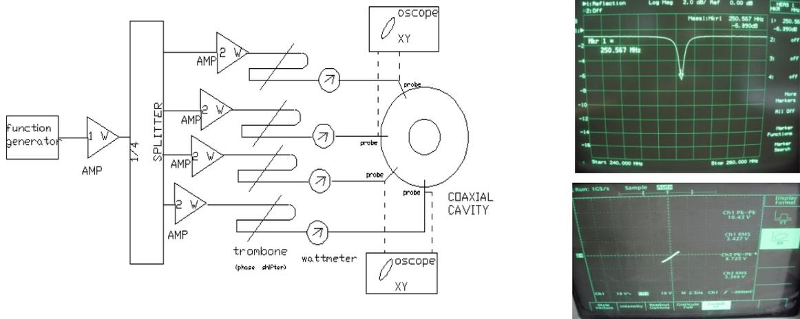
**Fig 24.** Schematic of the circuit with four input ports (left) and some measuring result (right).
