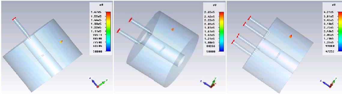
**Fig 22.** The effect of increasing number of ports on the electron beam energy in an accelerator cavity.
