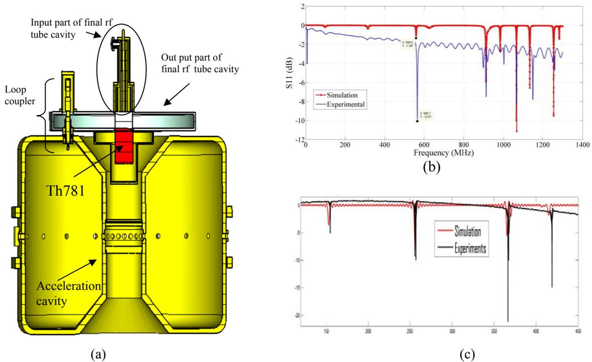
**Fig10.** (a)Section cut-view of the acceleration cavity showing location of the tube. (b)Comparison of impedance matching and return loss for the input and ( c)output ports of a rf tube cavity .
