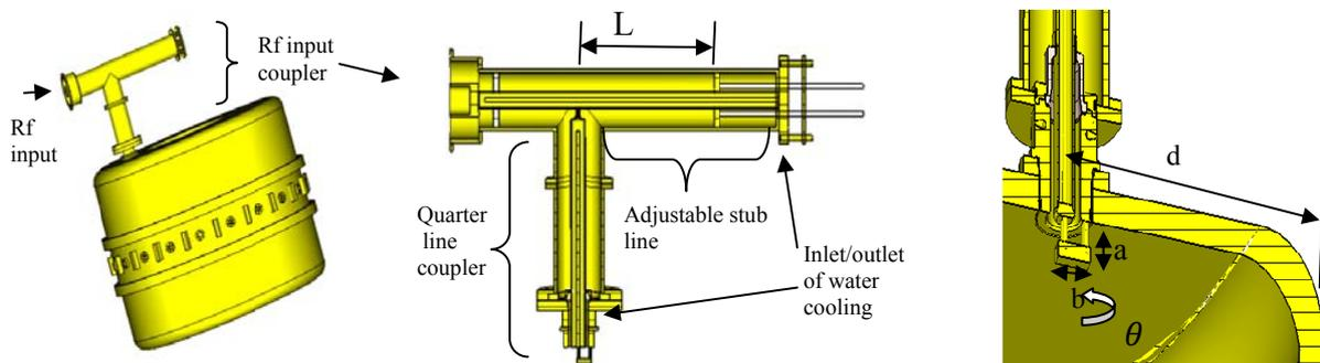
**Fig 16.** Section-cut view of the designed high power coupler and its position on the acceleration cavity
