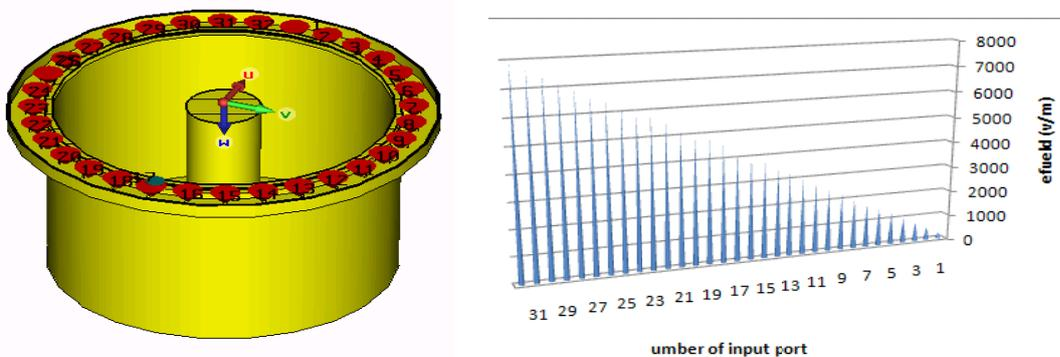
**Figure 27.** An acceleration cavity with 32 amplifier modules and the effect of number of modules on distribution of the electric field inside the acceleration cavity.
