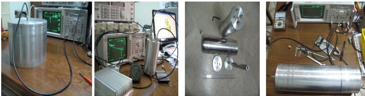
**Fig19.** Example of the power combiners designed and built.
