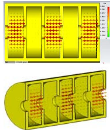
**Fig 5.**  $\pi/2$  resonance mode in a five-cell acceleration module.
