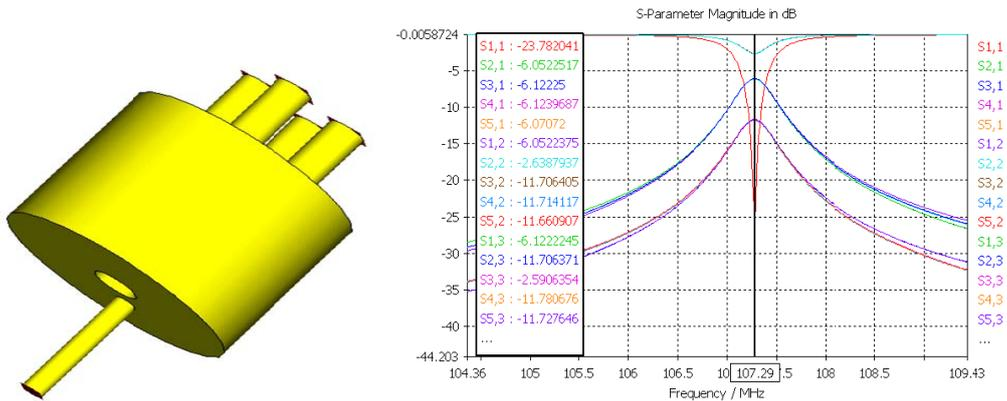
**Fig 20.** Power combiner with four inputs and one output with dimensions equal to those of a Rhodotron acceleration cavity.
