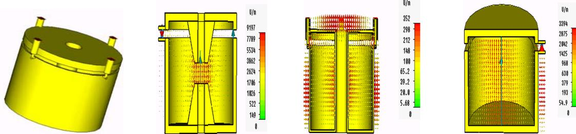
**Fig 25.** Several cavities with slit excited
