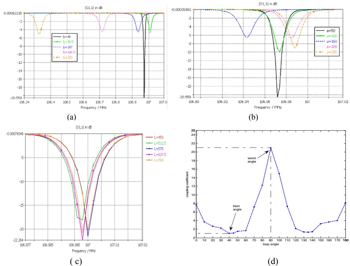
**Fig 12.** Effects of (a) coupler location on return loss, (b) coupler dimensions on return loss, (c) loop angle on coupling coefficient, and (d) the length of loop on resonance frequency.
