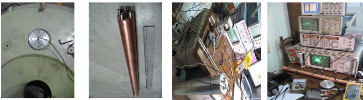
**Fig 23.** Several coaxial cavities built to perform tests.
