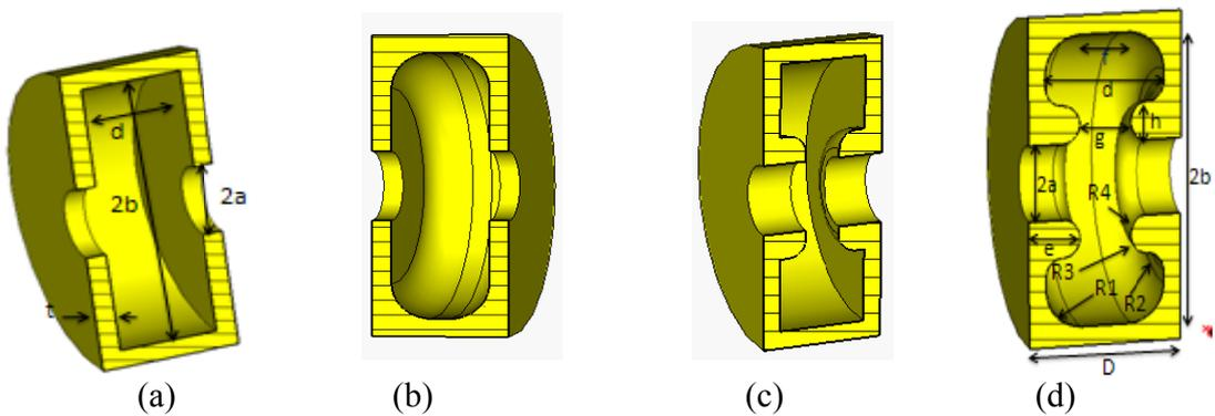
**Fig2.** Various shapes of a pill box cavity, from left to right: (a) simple pill box cavity (b) spherical pill box cavity (c) simple pill box cavity with nose, and (d) spherical pill box cavity with nose
