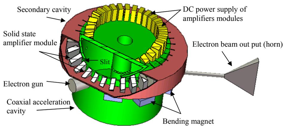
**Fig 28.** The new designed accelerator designed including solid state amplifier and slit cavity concepts.
