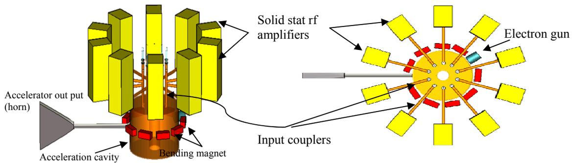
**Fig18.** Schematic sketch of design of the multiple input couplers to acceleration cavity.
