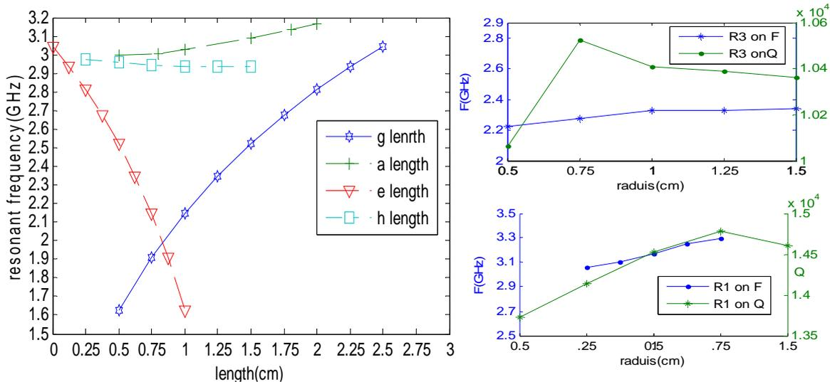
**Fig 4.** Effects of changing dimensions of cavity on frequency and quality factor.
