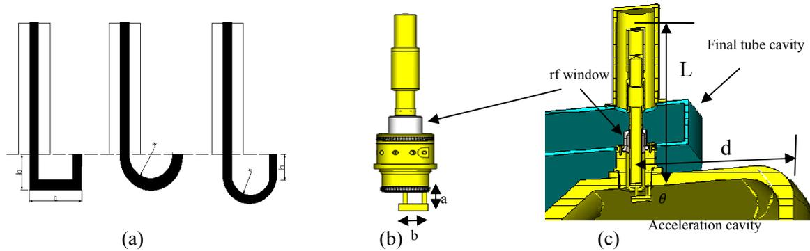
**Fig 11.**(a) Three types of couplers studied.(b) Cross-section view of the coupler and (b) location of the coupler inside the acceleration cavity
