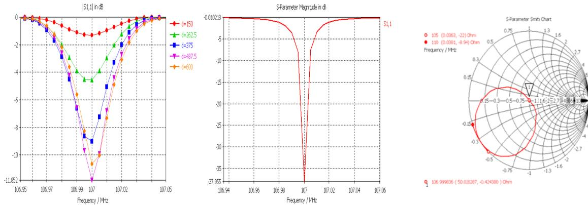
**Fig17.** The effects of different dimensional parameters of the designed coupler on (a) return loss and (b) impedance matching.
