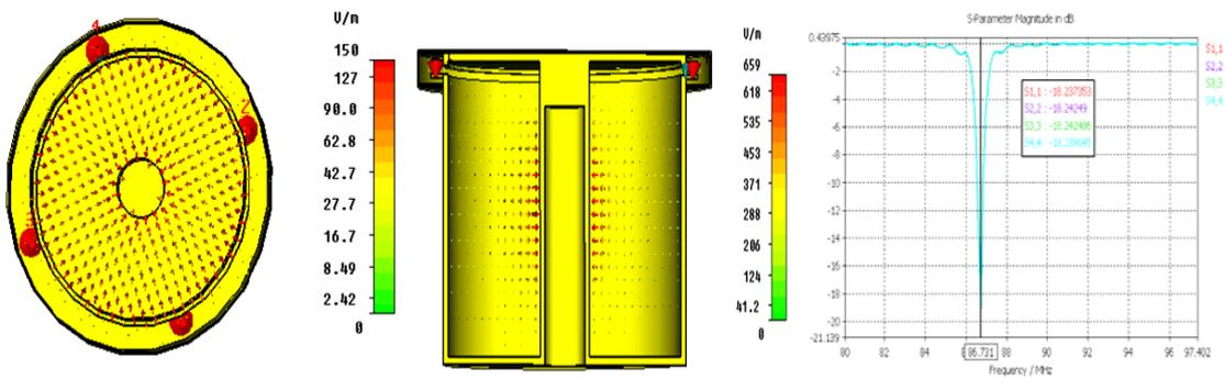
**Fig 26.** Return loss and electrical field calculated from numerical simulations for a coaxial acceleration cavity with direct connection of ports and using the secondary cavity.
