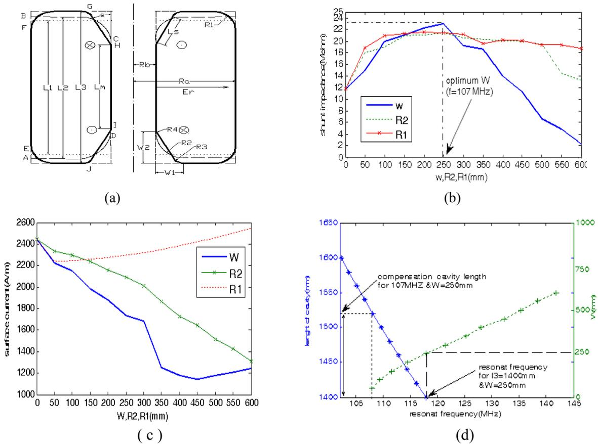
**Fig 9.** (a) Different shapes of an acceleration cavity. (b) The effects of dimensions on surface flow, (c) shunt impedance, and (d) resonant frequency.
