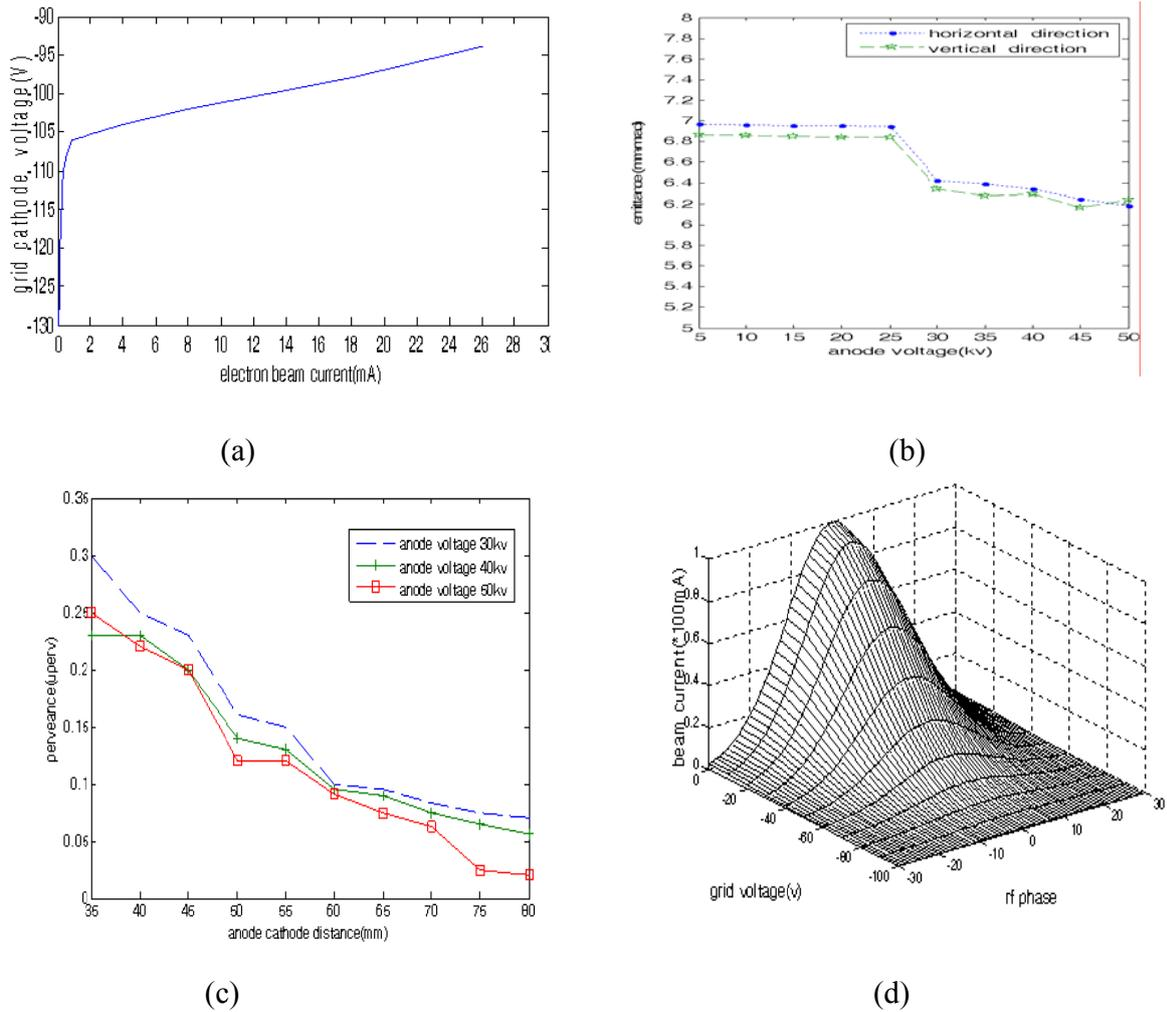
**Fig 8.** Results from the numerical simulations: (a) the effect of grid-to-cathode voltage on the electron beam current, (b) relation between anode voltage and emittance, (c) relation between anode-cathode distance and perveance, and (d) relation between RF phase and grid-to-voltage and the beam current.
