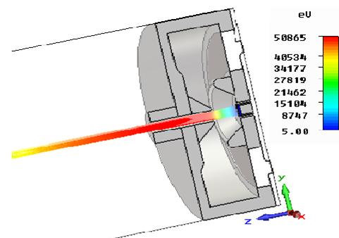
**Fig7.** Pattern of cathode and anode cavity and the produced beam
