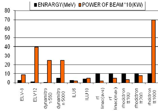
**Fig1.** Comparison of different industrial accelerators in terms of energy and power of the beam.
